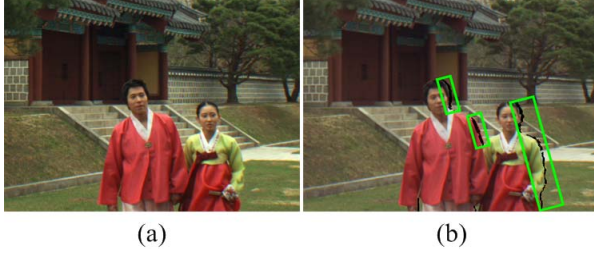
Fig. 1. An example of disoccluded areas. (a) Original image; (b) Synthesized image with distortions marked by green boxes.
